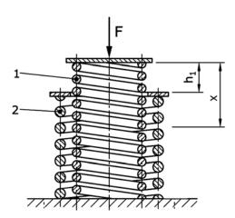
a) to be determined: spring rate  $c_2$  of spring 2, if  $c_1$ =12 N/mm is given for spring 1. [36 N/mm]
