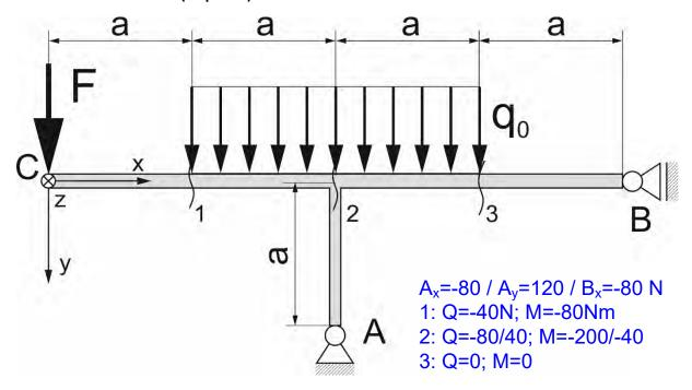
A beam is mounted in point B and, via support, in point A. The load F acts in point C against the beam. Additionally the line load  $q_o$  acts in the middle of the beam.
